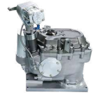
Hydrostatic Steering Unit (KAAV I Amphibious Vehicle)
